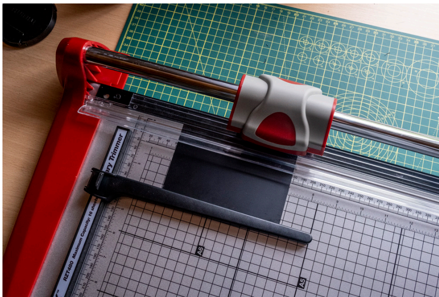
Cutting tintype plates to size (allow 1mm all around clearance to inside of insert – i.e. 126mm x 97mm)
