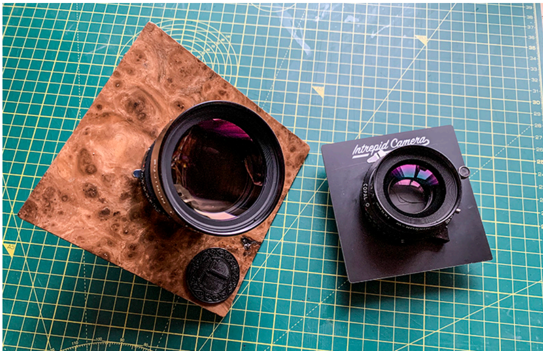
Note the 10x8 lens board and 300mm lens on the left and 5x4 lens board on the right with 150mm lens. Both lenses are Copal 0
